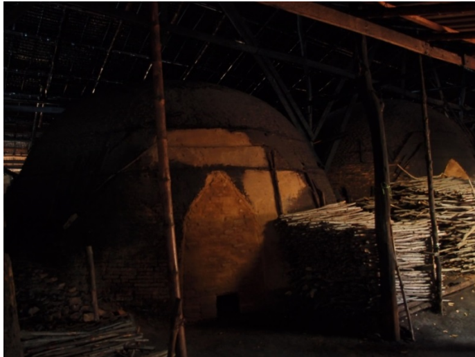
Photo⑥-2 : Dome-shaped charcoal kiln
